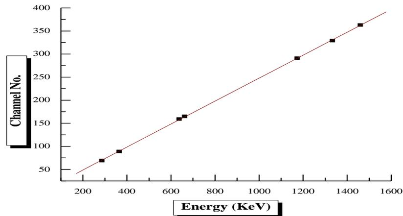
Figure (1) Energy Calibration for WBC.
