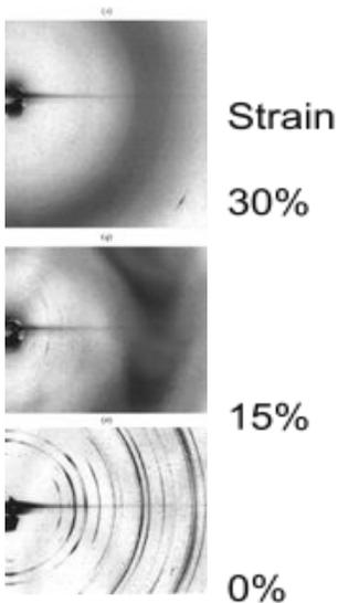
◀ **Fig.4.** SAXS images using a tensometer in BIGDIFF.
