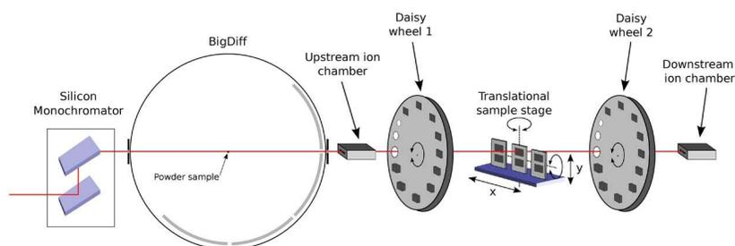
◀ **Fig.8.** Schematic diagram of the XERT technique.
