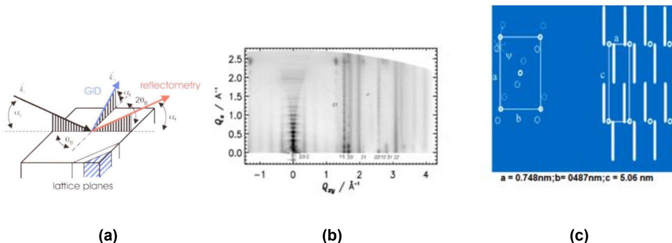
**Fig.6** (a) Schematic diagram illustrating the processes of XRR and GID.
