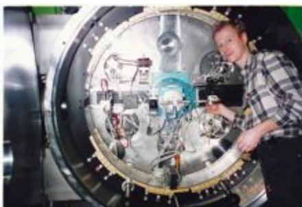
Shown in Fig.1 are the vacuum vessel, the Huber dual axis diffractometer base with motor-encoders on both axes (note that the axis of the diffractometer had to be located exactly on the axis of the film cassette (573mm radius)), specimen spinning stage (optional), the imaging plate holder. Of course, there are precision mounting rails, feed-throughs for electrical cables and so on.
