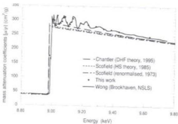
◀ **Fig.7** XAFS spectra for copper and a comparison of how closely the theoretical values match the experimental values.
