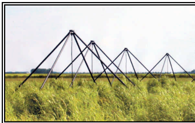
Figure 2. Elements of the LOFAR array: omni-directional antennae which are part of a phased array system. Reproduced from http://LOFAR.org .
