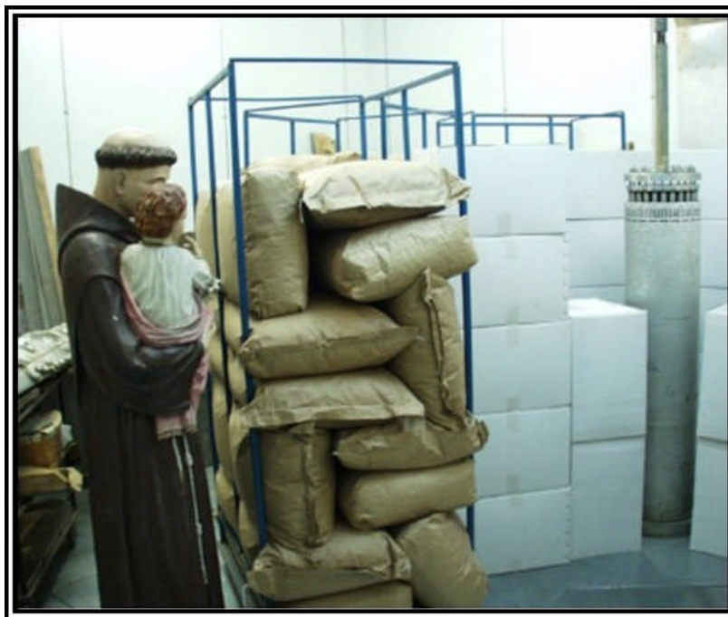
Figure 3. Panoramic ^{60}\text{Co} irradiation facility for radiation processing of food and the study of cultural heritage objects.
