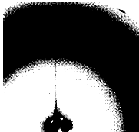
Figure 2 : Diffraction patterns from stressed elastomers (b) Fully loaded .. 320% strain
