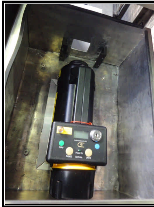
Fig. 3. The X-ray source in the source box, with the 3D camera removed. The beam defining aperture can be seen.
