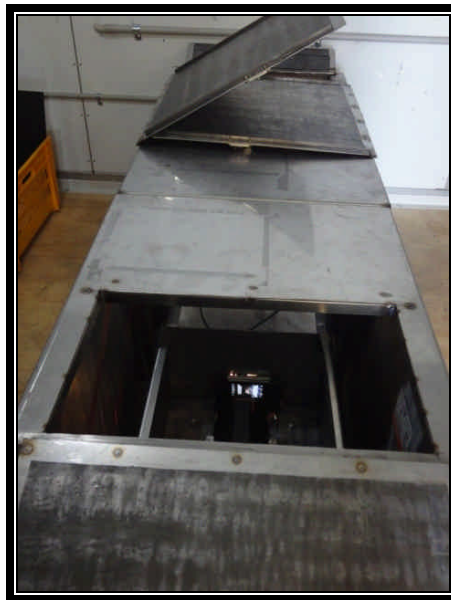
Fig. 2. X-ray enclosure showing the access doors for the X-ray source, the specimen stage, and the imaging plates. The X-ray source has been removed, and the camera inserted. The photographic image, presented on the viewing screen of the camera can be seen.
